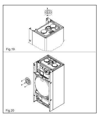
Using the screws and washers provided, secure the appliance onto the wall bracket and tighten with a suitable spanner. Seal the flue assembly to the wall using cement or a suitable alternative that will provide satisfactory weatherproofing. The exterior wall trim can now be fitted.
