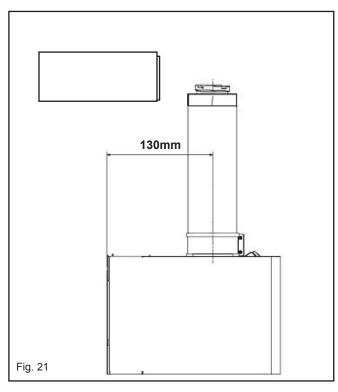
Fit the appropriate flashing plate to the roof and insert the vertical flue terminal through the flashing plate from the outside, ensuring that the collar on the flue terminal fits over the flashing. The fixing holes for the wall-mounting bracket should now be drilled and plugged, an 'appropriate type and quantity of fixing should be used to ensure that the bracket is mounted securely. Once the bracket has been secured to the wall, mount the appliance onto the bracket.
