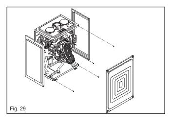
section 4.7.1 and drain the water content from the appliance via the drain valve. Ensure some water absorbent cloths are available to catch any residual water that may drip from the appliance or removed component. Undertake a complete commissioning check as detailed in section 5, after replacing any component. ALWAYS TEST FOR GAS TIGHTNESS IF ANY GAS CARRYING COMPONENTS HAVE BEEN REMOVED OR DISTURBED.
